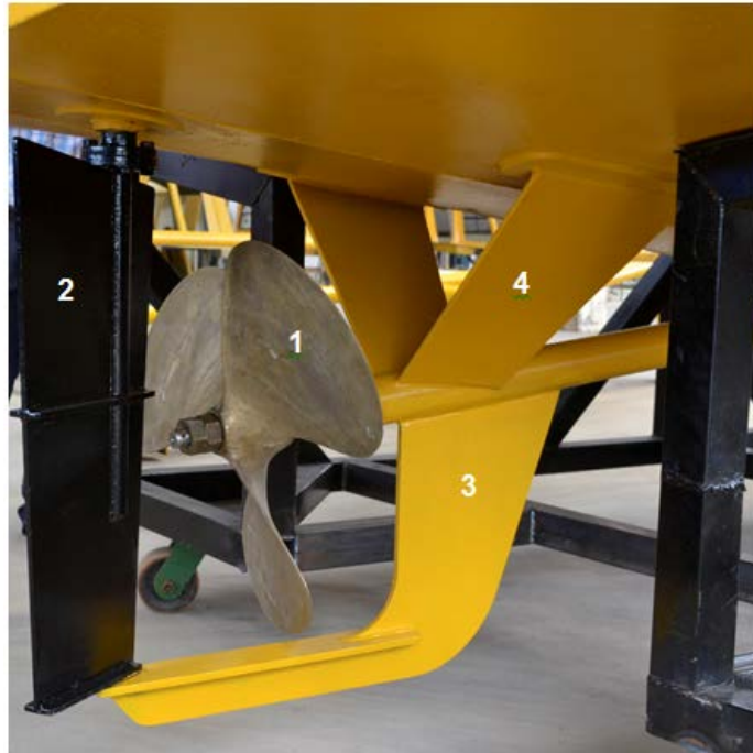
Figure 2: (1) Propeller, (2) rudder, (3) skeg and (4) propeller shaft bracket
