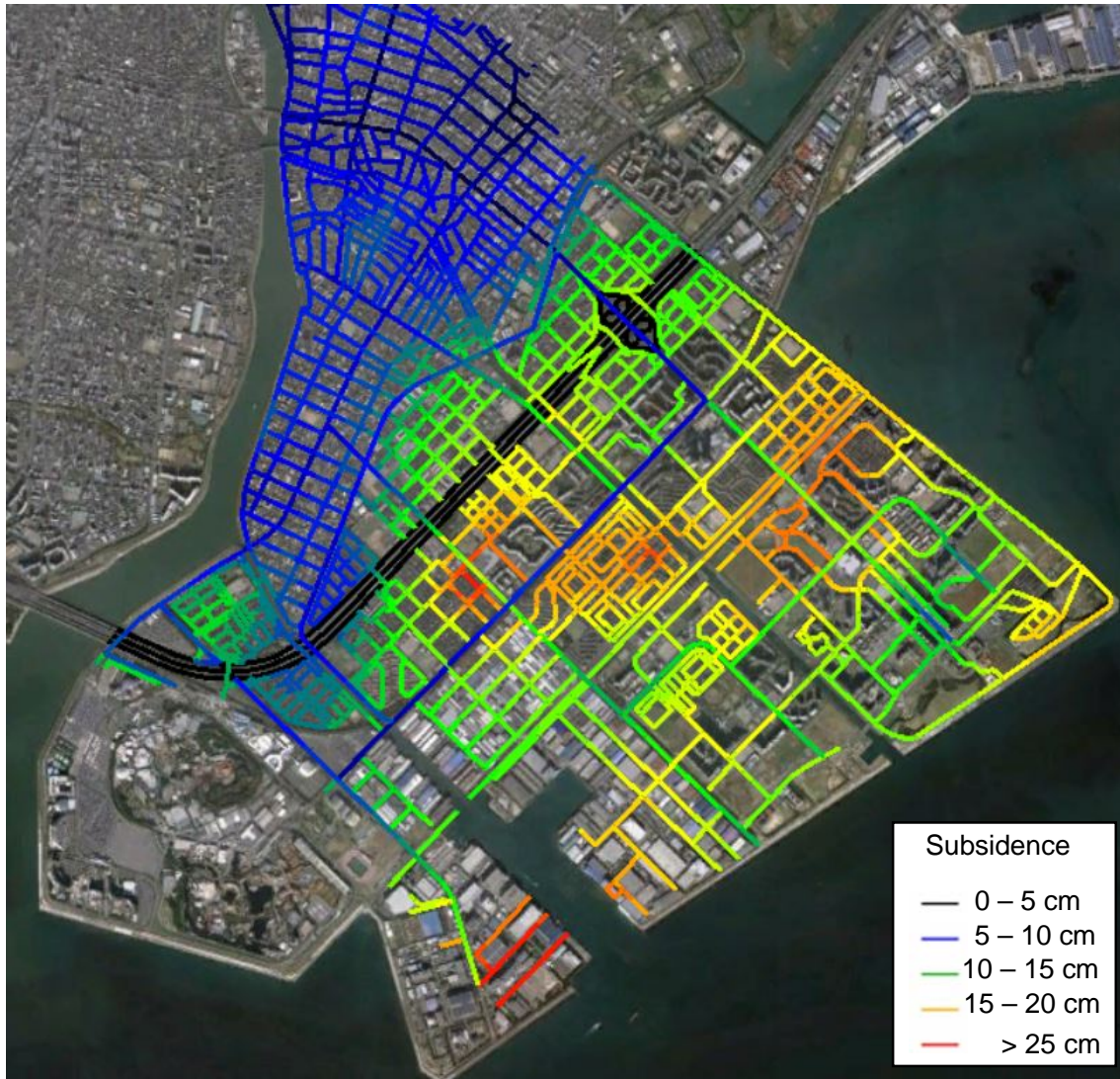
Figure 7 Estimated risk of road subsidence in Urayasu for a scenario earthquake on the scale of the 2011 Great East Japan Earthquake (Kajihara et al., 2015)
