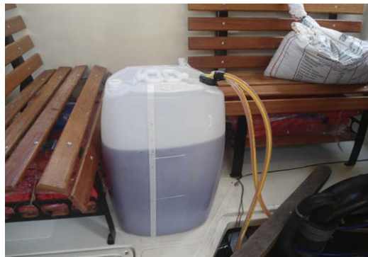
Figure 23: External fuel tank at diesel boat
