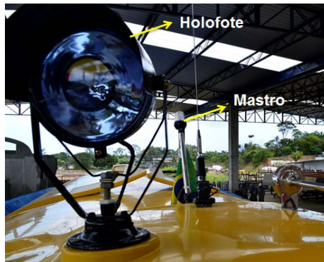
Figure 5: Installation of searchlight and mast with navigation light.
