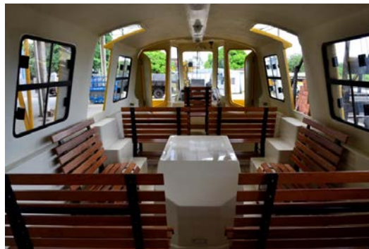
Figure 11: Internal aspect of bridge-house and boards attached to the roof and benches already assembled in the boat school big (view from fore).
