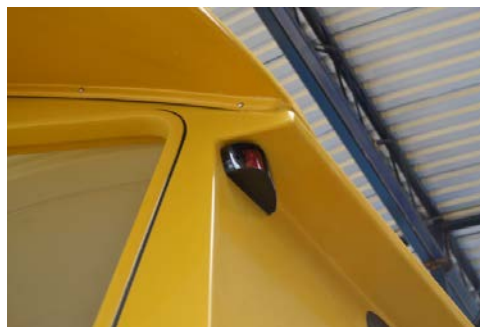
Figure 6: Port navigation light
